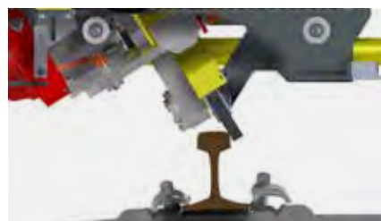
Maximum swivelling range: 32° in both directions with grinding disc module
