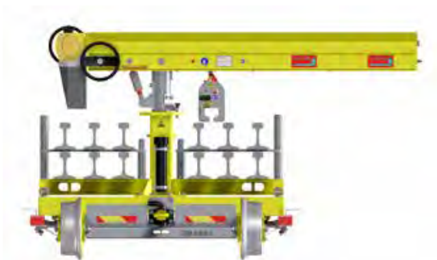
Loading diagram with 12 rails max. on 2 levels
