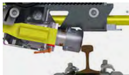
Maximum swivelling range 32° external and 80° internal
