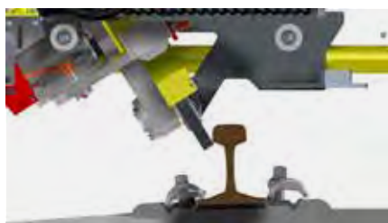
Maximum swivelling range: 32° in both directions with grinding disc module
