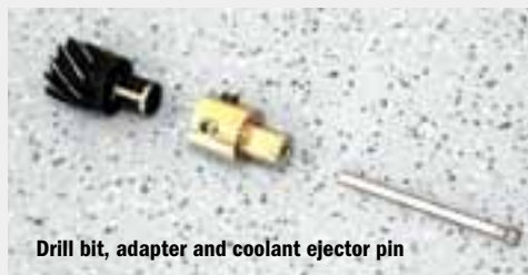
Adapter and 13 mm spiral drill bit
