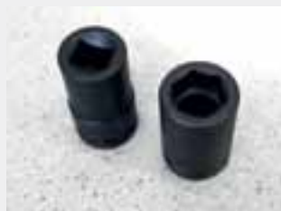
Socket rect. 24 x 28 for rectangular, socket A/F 39 for hexagonal
